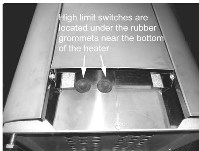
Location of High Limits: Press rubber grommets to reset buttons underneath.
