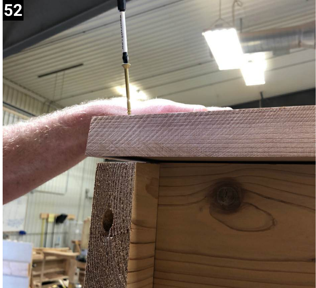
52 Put flush to the back and secure down with a couple 3" screws.
