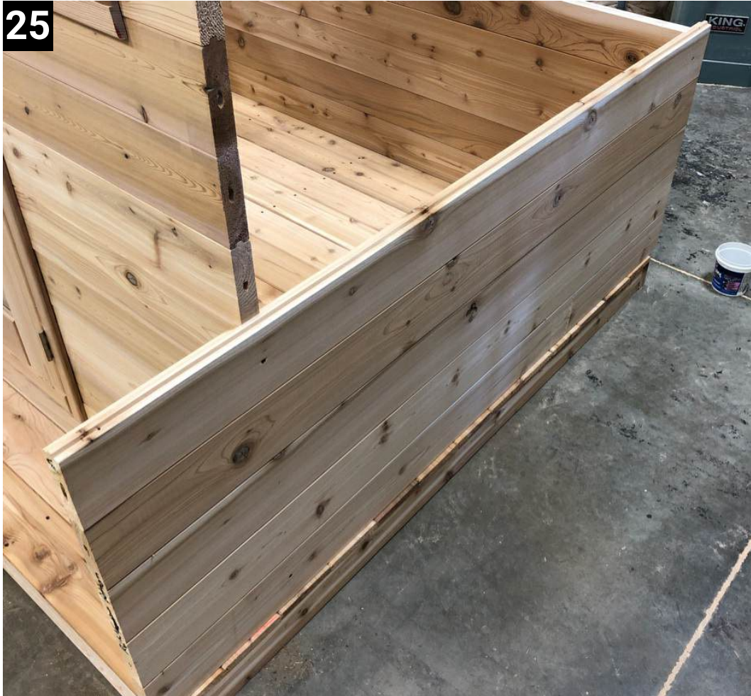
Slot the last bottom wall piece into the front and back walls
