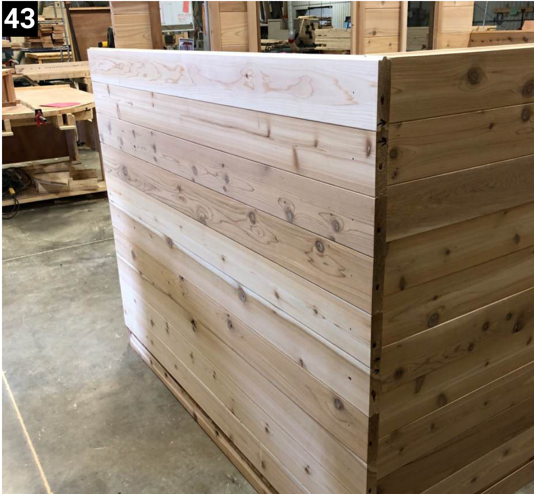
Attach the final middle wall piece
