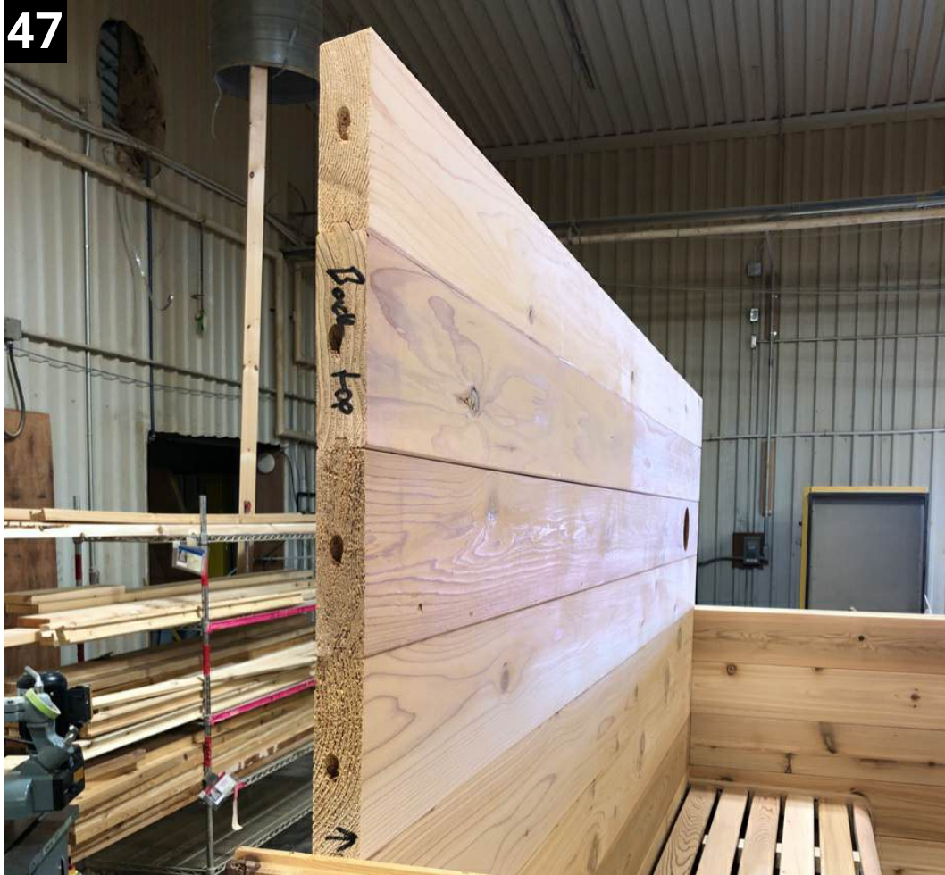
47 Attach the back top piece, make sure arrows are facing forward
