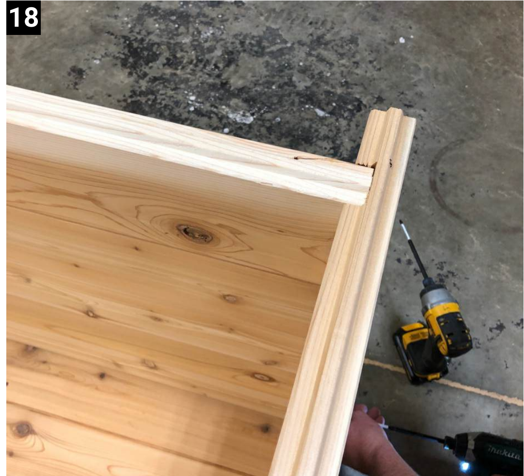
slot the other side of the back wall into the other side piece
