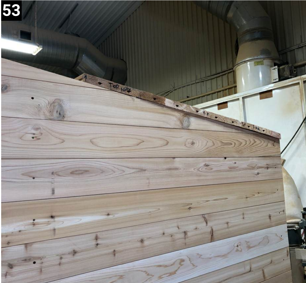
53 Place top middle piece on the roof and attach it to the top back piece with 4" screws
