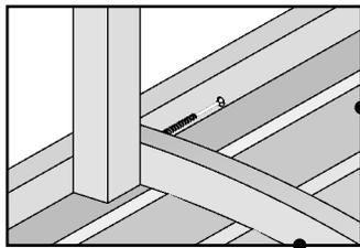
Pre-drill holes  $\varnothing 5/32"$  before screws.
