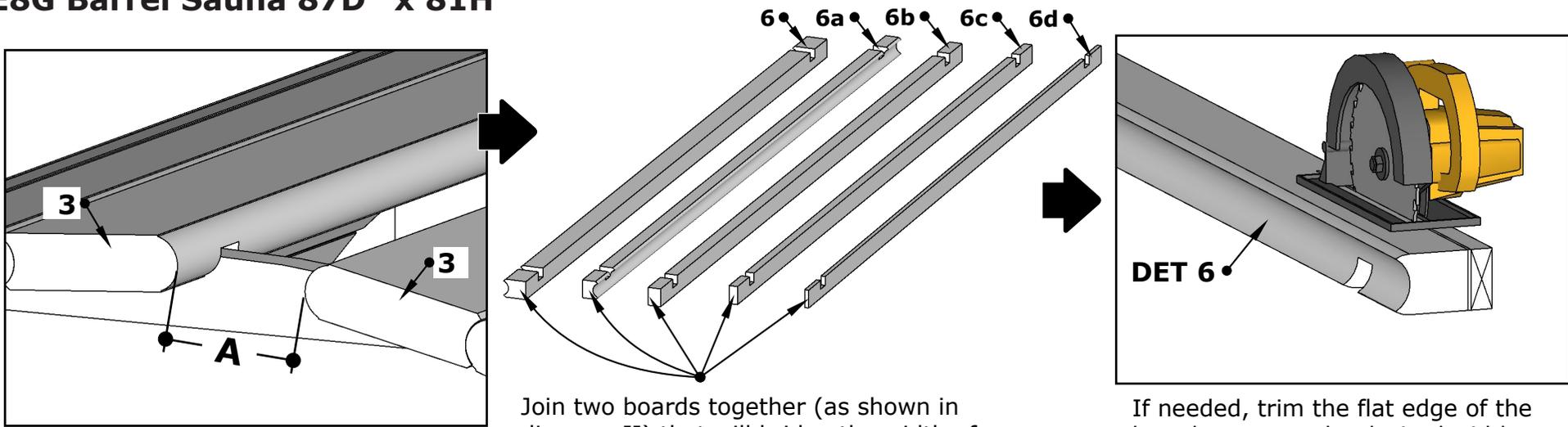
Join two boards together (as shown in diagram II) that will bridge the width of the "A" gap. It is recommended that the combined boards are approximately 1/4" wider than the gap.
