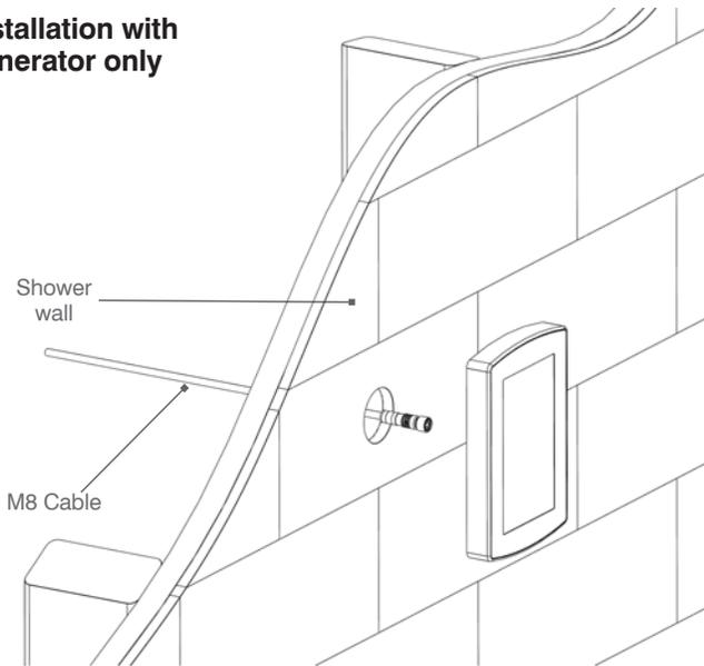
Route the M8 cable through the finished wall to the back side of the control. (The other end of the cable runs to the steam generator location.) NOTE: It is recommended to run the cable through electrical conduit. DO NOT STAPLE the cable!
